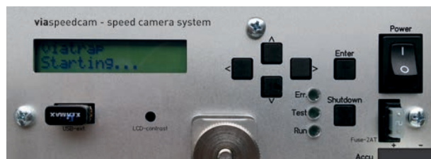
Camera unit and the control panel inside the battery box.
