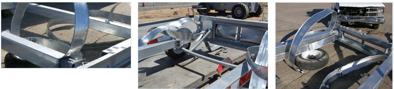
Figure 8 (left). Bursting of the energy-absorbing tube. Figure 9 (centre). Damage from a medium-speed impact. Figure 10 (right). Damage from a high-speed impact.
