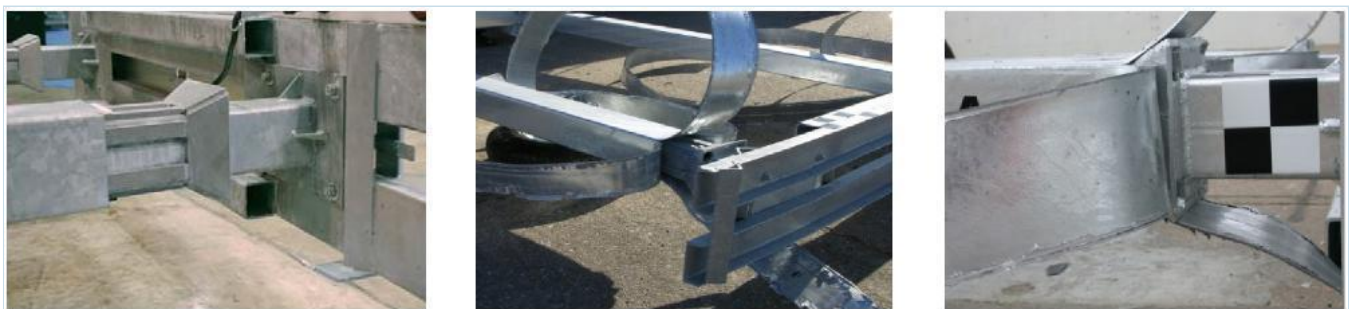
Figure 2. The bursting process. Left: tapered and over-sized mandrel inserted into the energy-absorbing tube. Centre: the mandrel cracks the tube at the corners and splits it into four flat straps of metal. Right: close-up of mandrel and energy-absorbing tube.
